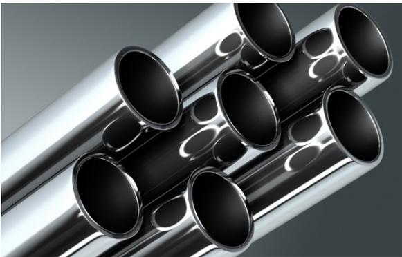
For applications with surface finish requirements well beyond the quality realized in a standard mill finish, PAC maintains an inventory of electropolished tubing (EP) in diameters ranging from 1/8" through 1". Through submersion in an electrically charged electrolyte solution bath, a smooth uniform surface is created by dissolving imperfections. This process removes any contamination on, or just below, the tube's surface and passivates it, bolstering the corrosion resistance of the steel.
