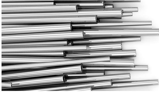
With the addition of molybdenum, grades 316 and 316L stainless steel were developed to offer improved corrosion resistance compared to alloy 304/L. The increased performance of this austenitic chromium-nickel stainless steel makes it better suited for environments rich in salt air and chlorides. Additionally, the low carbon content makes the alloy 316/L easy to weld.
