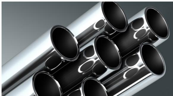
For applications with surface finish requirements well beyond the quality realized in a standard mill finish, PAC maintains an inventory of electropolished tubing (EP) in diameters ranging from 1/8" through 1". Through submersion in an electrically charged electrolyte solution bath, a smooth uniform surface is created by dissolving imperfections. This process removes any contamination on, or just below, the tube's surface and passivates it, bolstering the corrosion resistance of the steel.
